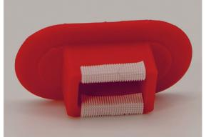
If the gap/cavity of the underside of the 3D model is narrow or small, as in the curved service desk and chairs, merely bridge the gap/open cavity with one continuous piece of hook strip.
